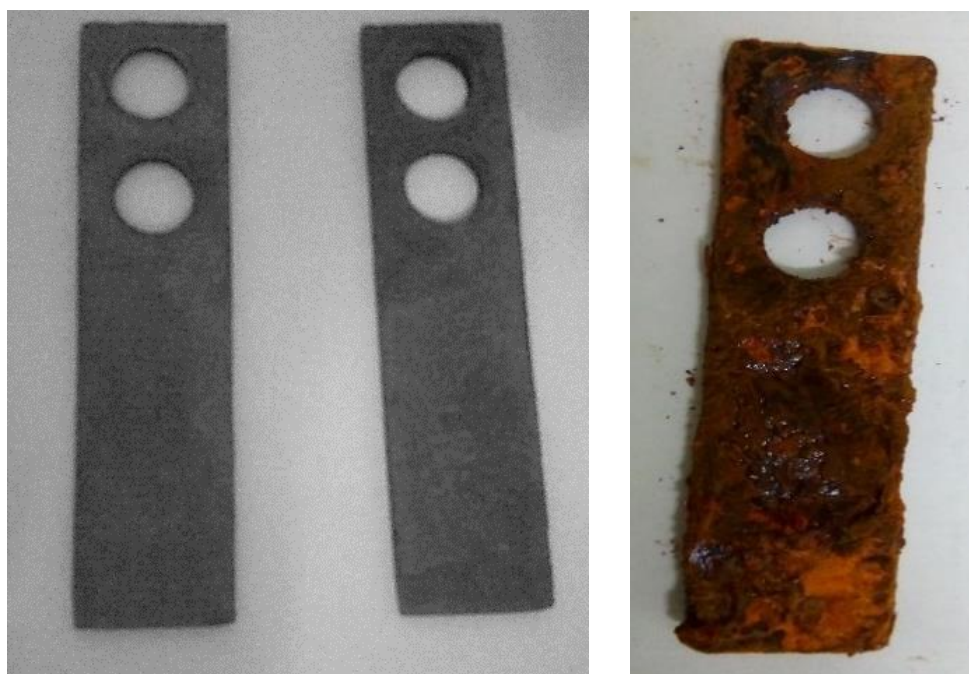
Figure 1. Metal plates – samples for corrosion rate measurements by the weight loss method.
