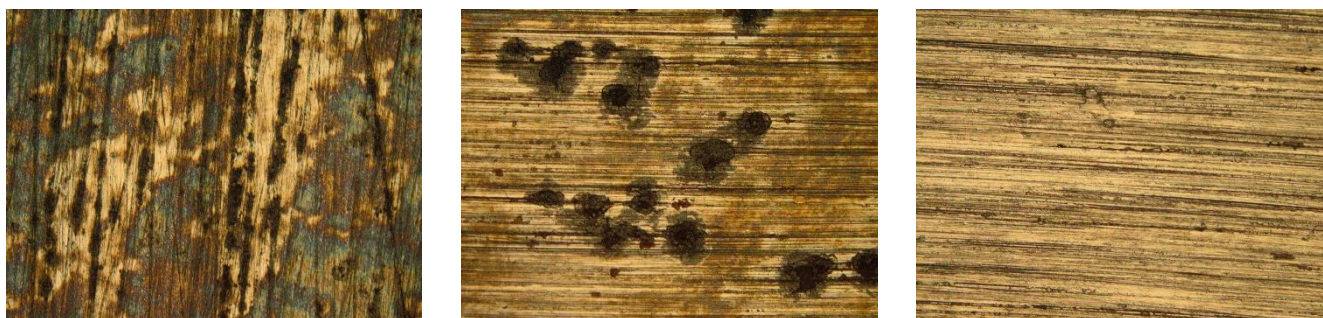
Figure 3. The R6M5 steel surface after removal of the corrosion products, from left to right: blank experiment, G-425, ES. Magnification \times 500 .
