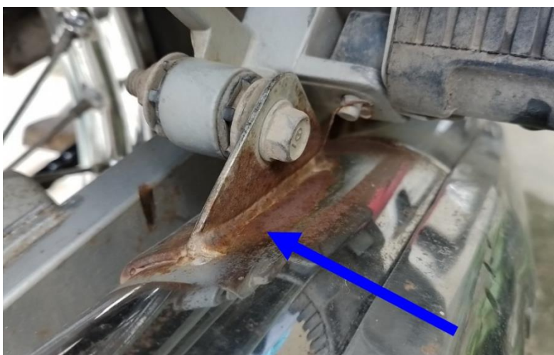
Figure 1. Welded motorbike exhaust joints that are corroded.
