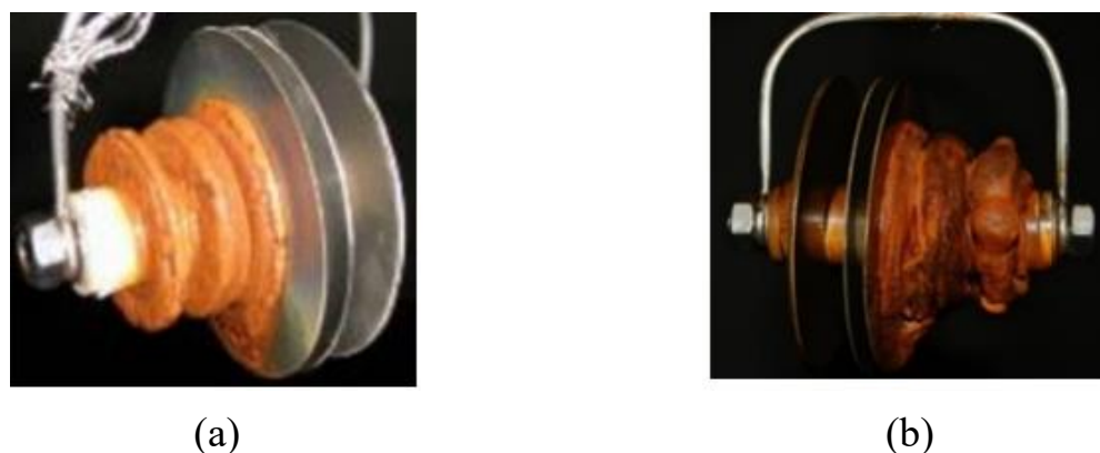
Figure 4. Visual examination results of coupons immersed in PUSPIPTEK water tank – vertical series. (a) 4 Months of immersion [25]; (b) 4 years of immersion.
