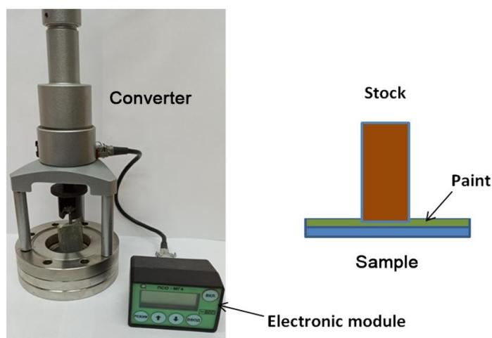
**Figure 1.** Electronic adhesion meter: PSO-MG4g.
