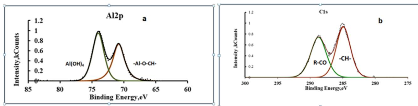
**Figure 8.** XPS spectra of Al2p (a) and C1s (b) for a modified conversion coating on AMg3 alloy.
