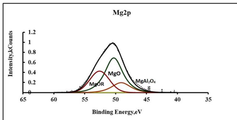
**Figure 4.** XPS spectra of Mg2p in a modified conversion coating on the MA20 alloy.
