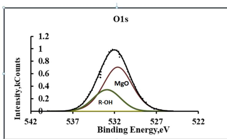
**Figure 6.** XPS-spectra of O1S oxygen in the modified conversion coating on the MA20 alloy.
