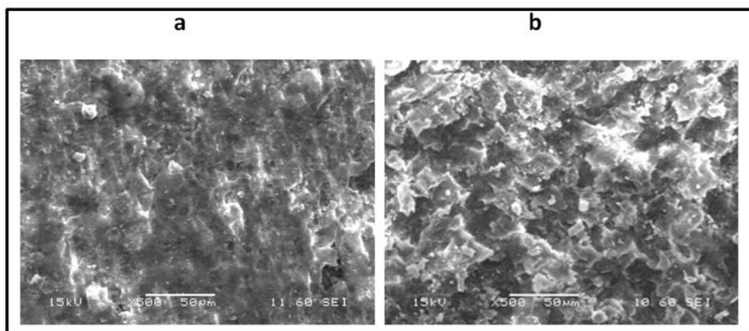
**Figure 3.** SEM images of the surface of the MA20 anodized alloy before (a) and after (b) modification with ethylene glycol.
