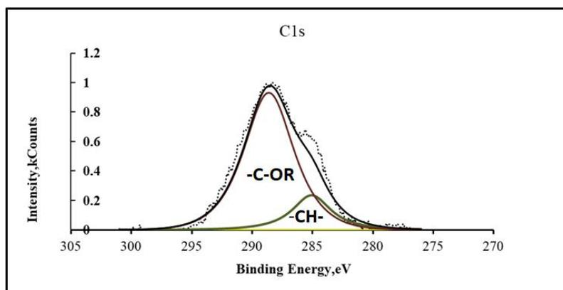
**Figure 5.** XPS spectra of C1s carbon in a modified conversion coating on the MA20 alloy.
