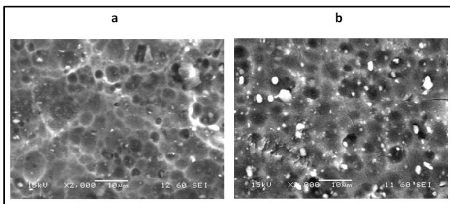
**Figure 7.** SEM images of the surface of the AMg3 conversion coating before (a) and after (b) modification with ethylene glycol.
