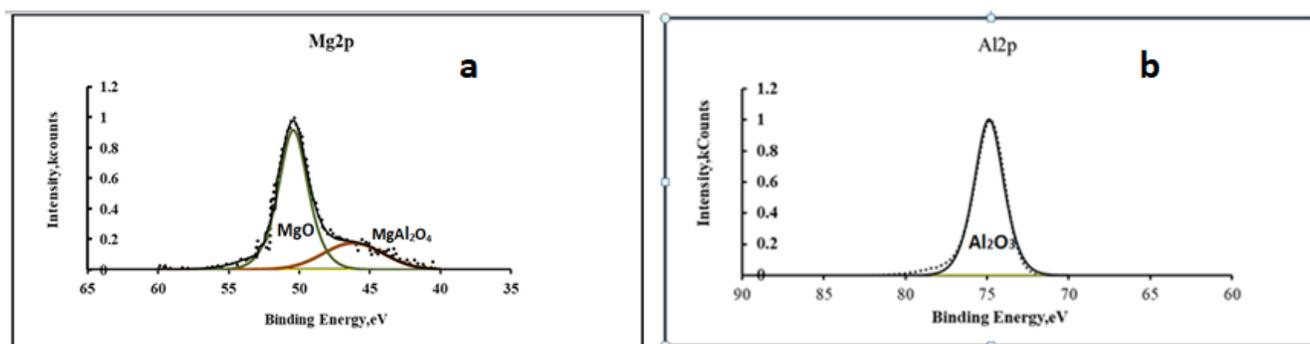
**Figure 2.** XPS spectra of Mg2p (a) and Al2p (b) in the MA20 conversion coating.
