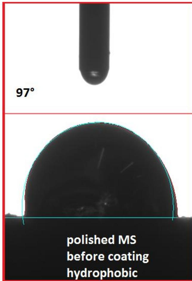
**Figure 17.** Contact angle of polished mild steel surface.
