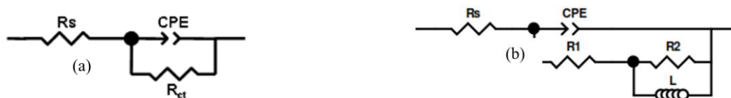
Figure 10. Model of the equivalent circuit for the steel/1 M HCl interface: (a) in the presence of Pyz1 and (b) in the presence of Pyz2 at 10^{-5} M.
