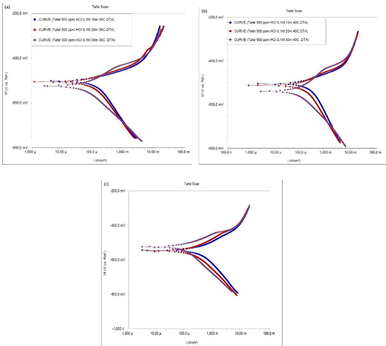
**Figure 7.** Tafel polarization curve of API 5L in HCl solution with various immersion times and 500 ppm PNLE inhibitor concentration at (a) 30°C, (b) 40°C, and (c) 50°C.
