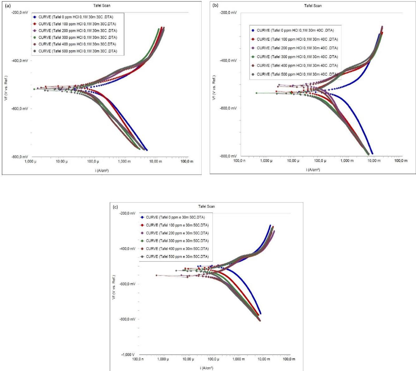
**Figure 5.** Tafel polarization curve of API 5L in HCl solution with various PNLE inhibitor concentrations at (a) 30°C, (b) 40°C, and (c) 50°C.
