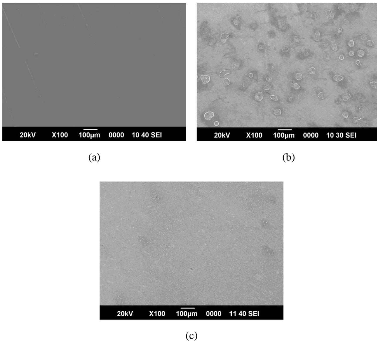
**Figure 8.** SEM image of API 5L (a) before immersing, (b) without inhibitor, and (c) with 500 ppm PNLE inhibitor in HCl solution.
