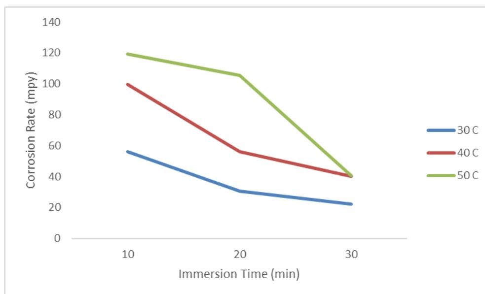
**Figure 6.** Corrosion rate vs immersion time.
