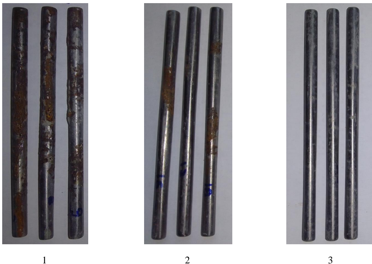
Figure 5. Appearance of reinforcing bars after 44 months of exposure of specimens with 3% sodium chloride in the tropics. 1 – samples containing no inhibitor, 2 – samples containing 1.5% inhibitor, 3 – samples containing 3% inhibitor.
