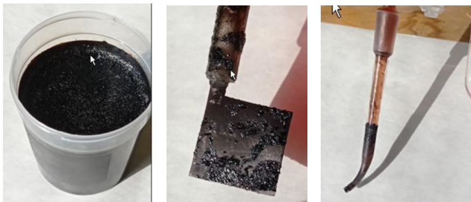
Figure 7. Photos of the cell, electrode and Luggin capillary after 1 month of exposure in a solution with 1 g/L CC.
