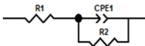
Figure 4. Electrical equivalent circuit used to fit the EIS data of the interface mild steel / 1 M HCl solution without and with investigated inhibitors.
