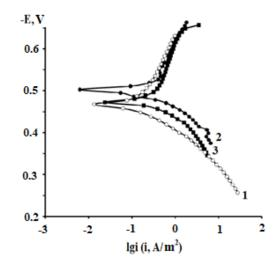
**Figure 2.** Potentiodynamic polarization curves of St3 steel in a 0.1 M NaCl solution in the absence of (1) and in the presence of ammonium sulfide 50 mg/L (2, 3) and 100 mg/L IFKhAN-114 (3).
