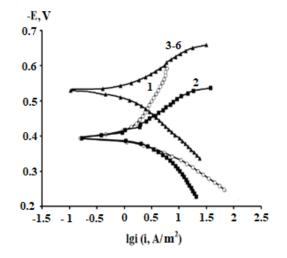
**Figure 1.** Potentiodynamic polarization curves of St3 steel in a 0.1 M NaCl solution in the absence (1) and in the presence of 50 mg/L of IFKhAN-114 (2–6). Duration of exposure of the electrode in the corrosive environments, h: 1, 2 - 0.25; 3 - 24; 4 - 48; 5 - 72; 6 - 98.
