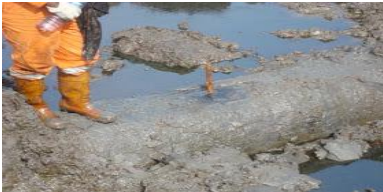
Figure 9. The pipeline after the leak had been stopped (by hammering a stick into the hole), showing apparent corrosion around the leak site. Source: Center for Environment, Human right and development www.sciencythoughts.blogs
