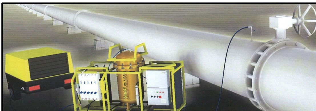
Figure 7. Mothaballing pipeline systems for applying DH-VCI (DVS-2) system.
