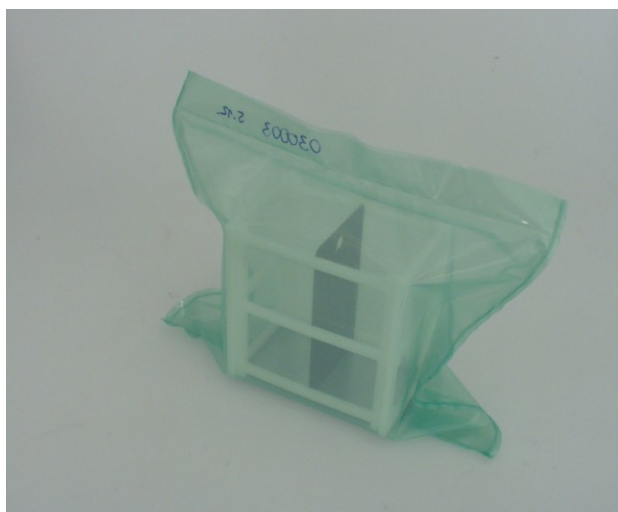
Figure 9. Model packages of the EXCOR internal “DIS” test.
