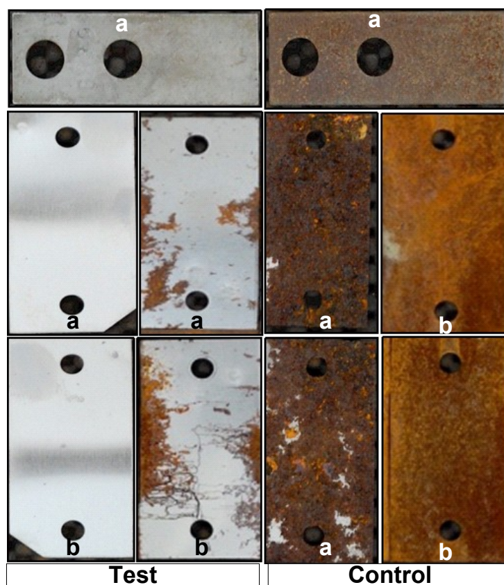
Figure 7. Corrosion conditions of the front (a) and the back (b) sides of the test and control coupons after one year field trial.
