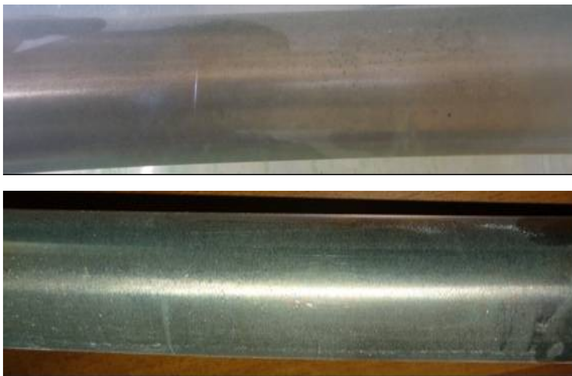
Figure 12. Absence of \text{CaCO}_3 deposits on the heat exchanger in the experiment with Dequest PB 11620 as inhibitor.
