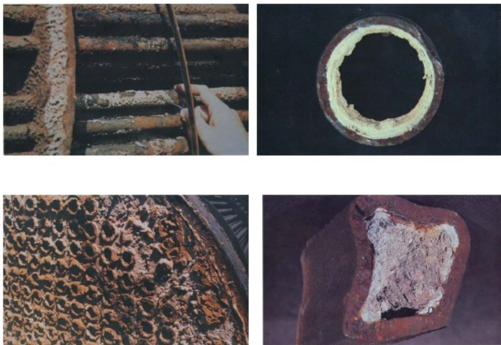
Figure 1. Scaled heat exchanger tube bundles (left images) and tubing (right images).
